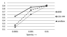
Figure 6: Ratio of in-memory MKL csrmm to BLAS-on-flash csrmm running times for  $(2^{20} \times 2^{17} \times 2^{12})$  sized instances and various values of sparsity. BLAS-on-flash uses a 8GB Program Cache. Each csrmm task uses 4 threads and the number of simultaneous tasks is determined by number of cores in the system.
