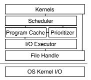
Figure 3: The BLAS-on-flash software stack.
