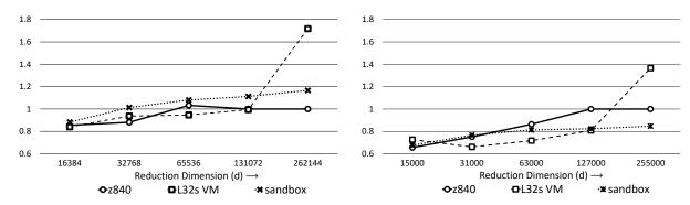
Figure 5: Ratio of in-memory MKL gemm to BLAS-on-flash gemm running times for 512-aligned (left) and unaligned (right) instances for various values of reduction dimension (d). The matrix dimensions are  $2^{15} \times d \times 2^{15}$  and  $31000 \times d \times 31000$  for the aligned and unaligned plots. BLAS-on-flash library has a 8GB Program Cache. gemm tasks in BLAS-on-flash library use 4 threads each. Program Cache budget determines the number of simultaneous tasks.
