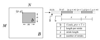
Figure 2:  $\langle b, \{l, s, n\} \rangle$  is an access specifier for block b of a flash-resident matrix B stored in Row-Major layout.
